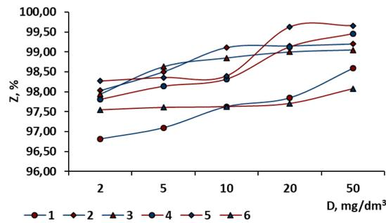
Figure 3. Dependence of oil removal from fresh (1, 2, 3) and salt (4, 5, 6) water ( $[H_{initial}] = 100 \text{ mg/dm}^3$ ) depending on the type of coagulant  $\text{Al}_2(\text{SO}_4)_3$  (1, 4),  $\text{Al}(\text{OH})_3$  (2, 5),  $\text{Al}(\text{OH})_2\text{Cl}$  (3, 6), and their doses ( in terms of  $\text{Al}_2\text{O}_3$ )
