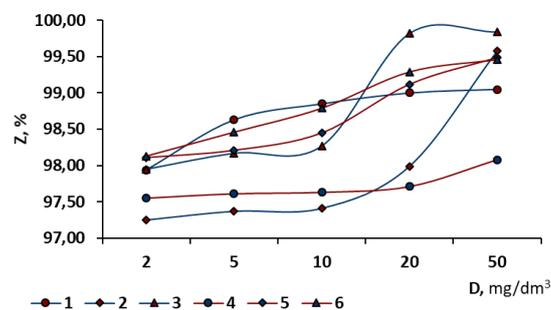
Figure 10. Dependence of oil removal from fresh (1, 2, 3) and salt (4, 5, 6) water ( $[H_{initial}] = 100 \text{ mg/dm}^3$ ) depending on the dose of  $\text{Al(OH)}_2\text{Cl}$  (in terms of  $\text{Al}_2\text{O}_3$ ) and the working concentration of the sorbent:  $0 \text{ mg/dm}^3$  (1, 4),  $50 \text{ mg/dm}^3$  (2,5),  $100 \text{ mg/dm}^3$  (3, 6)
