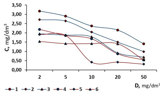
Figure 5. Change in the concentration of oil in fresh (1, 2, 3) and salt (4, 5, 6) water ( $[H_{initial}] = 100 \text{ mg/dm}^3$ ) depending on the dose of  $\text{Al}_2(\text{SO}_4)_3$  (in terms of  $\text{Al}_2\text{O}_3$ ) and the working concentration of the sorbent:  $0 \text{ mg/dm}^3$  (1, 4),  $50 \text{ mg/dm}^3$  (2,5),  $100 \text{ mg/dm}^3$  (3, 6)
