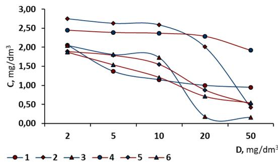
Figure 9. Change in the concentration of oil in fresh (1, 2, 3) and salt (4, 5, 6) water ( $[H_{initial}] = 100 \text{ mg/dm}^3$ ) depending on the dose of  $\text{Al(OH)}_2\text{Cl}$  (in terms of  $\text{Al}_2\text{O}_3$ ) and the working concentration of the sorbent:  $0 \text{ mg/dm}^3$  (1, 4),  $50 \text{ mg/dm}^3$  (2,5),  $100 \text{ mg/dm}^3$  (3, 6)
