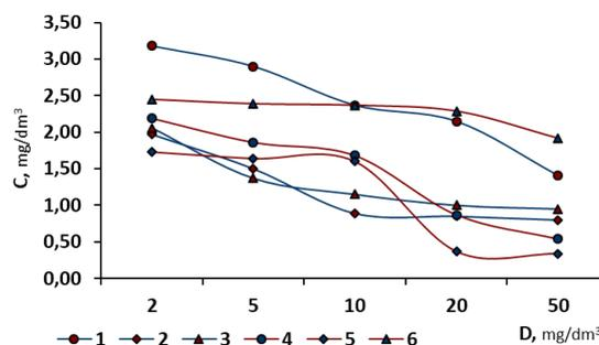
Figure 2. Change in the concentration of oil in fresh (1, 2, 3) and salt (4, 5, 6) water ( $[H_{initial}] = 100 \text{ mg/dm}^3$ ) depending on the type of coagulant  $\text{Al}_2(\text{SO}_4)_3$  (1, 4),  $\text{Al}(\text{OH})_3$  (2, 5),  $\text{Al}(\text{OH})_2\text{Cl}$  (3, 6), and their doses (in terms of  $\text{Al}_2\text{O}_3$ )
