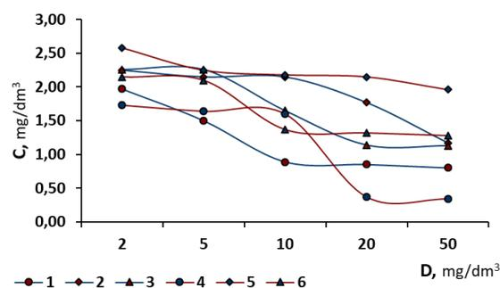
Figure 7. Change in the concentration of oil in fresh (1, 2, 3) and salt (4, 5, 6) water ( $[H_{initial}] = 100 \text{ mg/dm}^3$ ) depending on the dose of  $\text{Al}(\text{OH})_3$  (in terms of  $\text{Al}_2\text{O}_3$ ) and the working concentration of the sorbent:  $0 \text{ mg/dm}^3$  (1, 4),  $50 \text{ mg/dm}^3$  (2,5),  $100 \text{ mg/dm}^3$  (3, 6)
