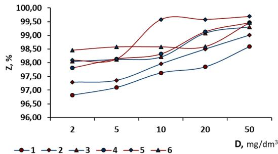
Figure 6. Dependence of oil removal from fresh (1, 2, 3) and salt (4, 5, 6) water ( $[H_{initial}] = 100 \text{ mg/dm}^3$ ) depending on the dose of  $\text{Al}_2(\text{SO}_4)_3$  (in terms of  $\text{Al}_2\text{O}_3$ ) and the working concentration of the sorbent:  $0 \text{ mg/dm}^3$  (1, 4),  $50 \text{ mg/dm}^3$  (2,5),  $100 \text{ mg/dm}^3$  (3, 6)
