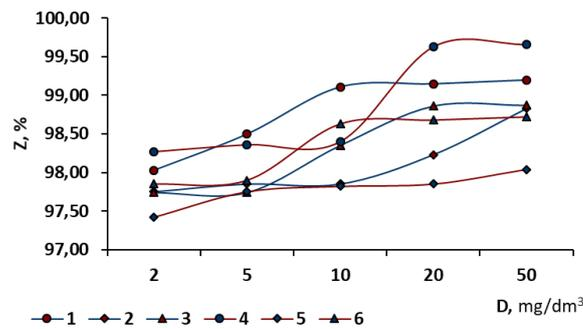
Figure 8. Dependence of oil removal from fresh (1, 2, 3) and salt (4, 5, 6) water ( $[H_{initial}] = 100 \text{ mg/dm}^3$ ) depending on the dose of  $\text{Al(OH)}_3$  (in terms of  $\text{Al}_2\text{O}_3$ ) and the working concentration of the sorbent:  $0 \text{ mg/dm}^3$  (1, 4),  $50 \text{ mg/dm}^3$  (2,5),  $100 \text{ mg/dm}^3$  (3, 6)
