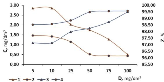
Figure 4. Dependence of residual oil concentration in fresh (1, 2, 3) and salt (4, 5, 6) water ( $[H_{initial}] = 100 \text{ mg/dm}^3$ ) and degree of oil removal from fresh (3) and salt (4) waters on the sorbent dose
