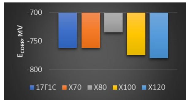
Fig. 3. Comparison of corrosion potential E_{cor} for different pipe steels
