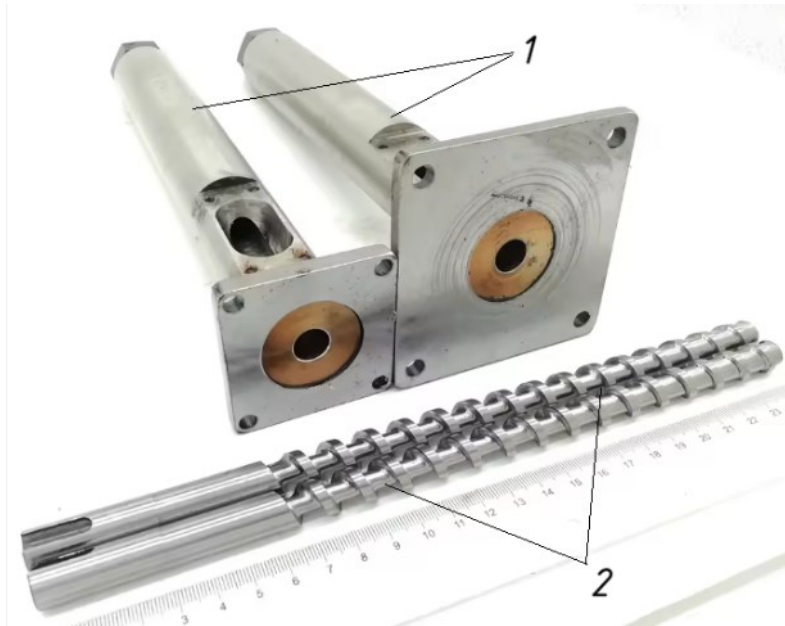
Fig. 2. Extruder barrel: 1-barrel; 2-screw [5]
